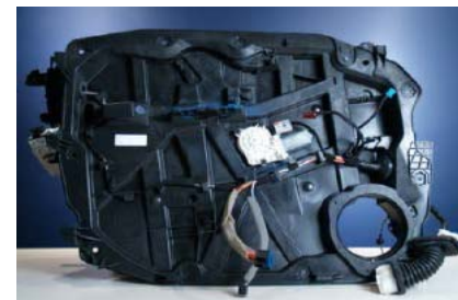
Door module PP + long GF → PP + short GF
