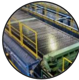
Membrane process chlor-alkali electrolysis
