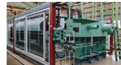
Ion-exchange membrane chlor-alkali electrolysis process
