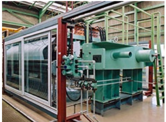
Ion-exchange membrane process for chlor-alkali electrolysis
