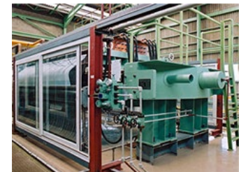
Ion-exchange membrane process for chlor-alkali electrolysis
