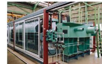
Ion-exchange membrane chlor-alkali electrolysis process
