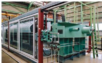
Ion-exchange membrane chlor-alkali electrolysis process
