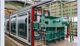
Ion-exchange membrane chlor-alkali electrolysis process
