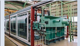
Ion-exchange membrane chlor-alkali electrolysis process
