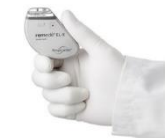
Implantable central sleep apnea (CSA) treatment device
