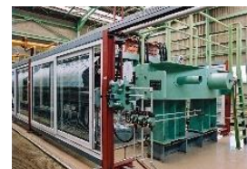
Ion-exchange membrane process chlor-alkali electrolysis Reducing power consumption in electrolysis
