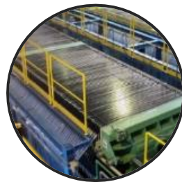
Membrane process chlor-alkali electrolysis
