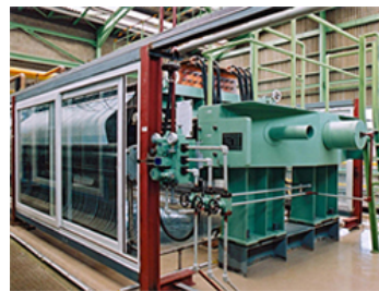
> Ion-exchange membrane process for chlor-alkali electrolysis
